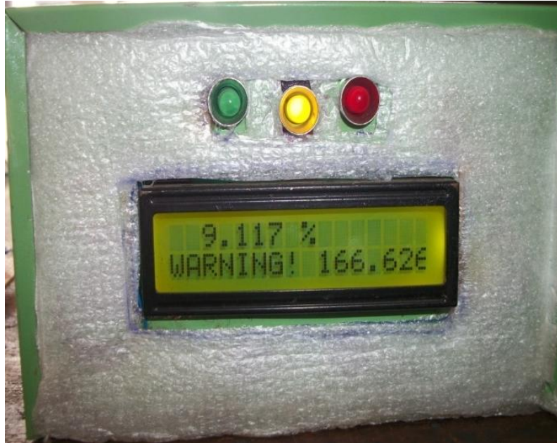
Figure 3. Overall view of the developed processing and display unit.
